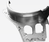
4.3 PANEL ASSEMBLY REAR WHEEL HOUSING OUTER
