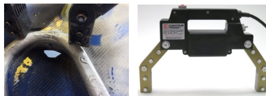
Sample image of NDT inspection using magnetic particle method (left image) and the equipment used (right image)
