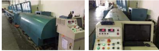
400-ton tensile testing machine
