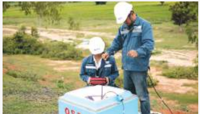
Open End Standpipe Piezometer Installation
