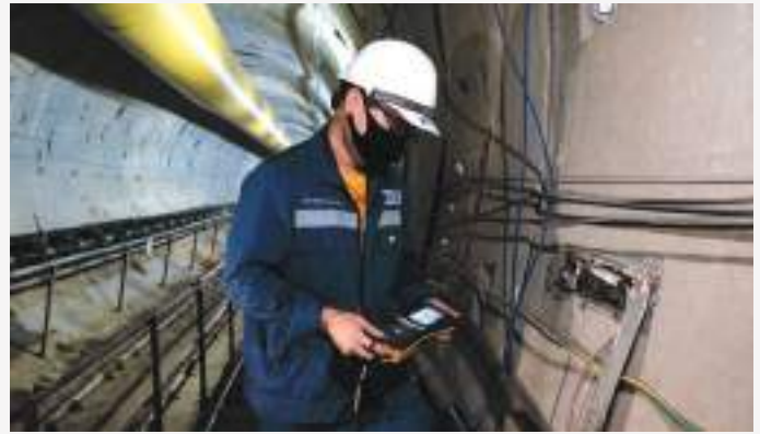
Total Pressure Cell Monitoring in Tunnel
