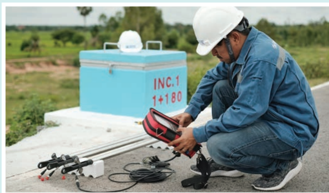
In-place Inclinometer
