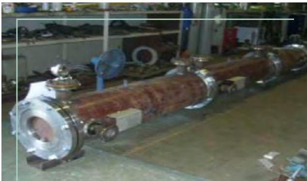
Heat Pipe Fabrication
