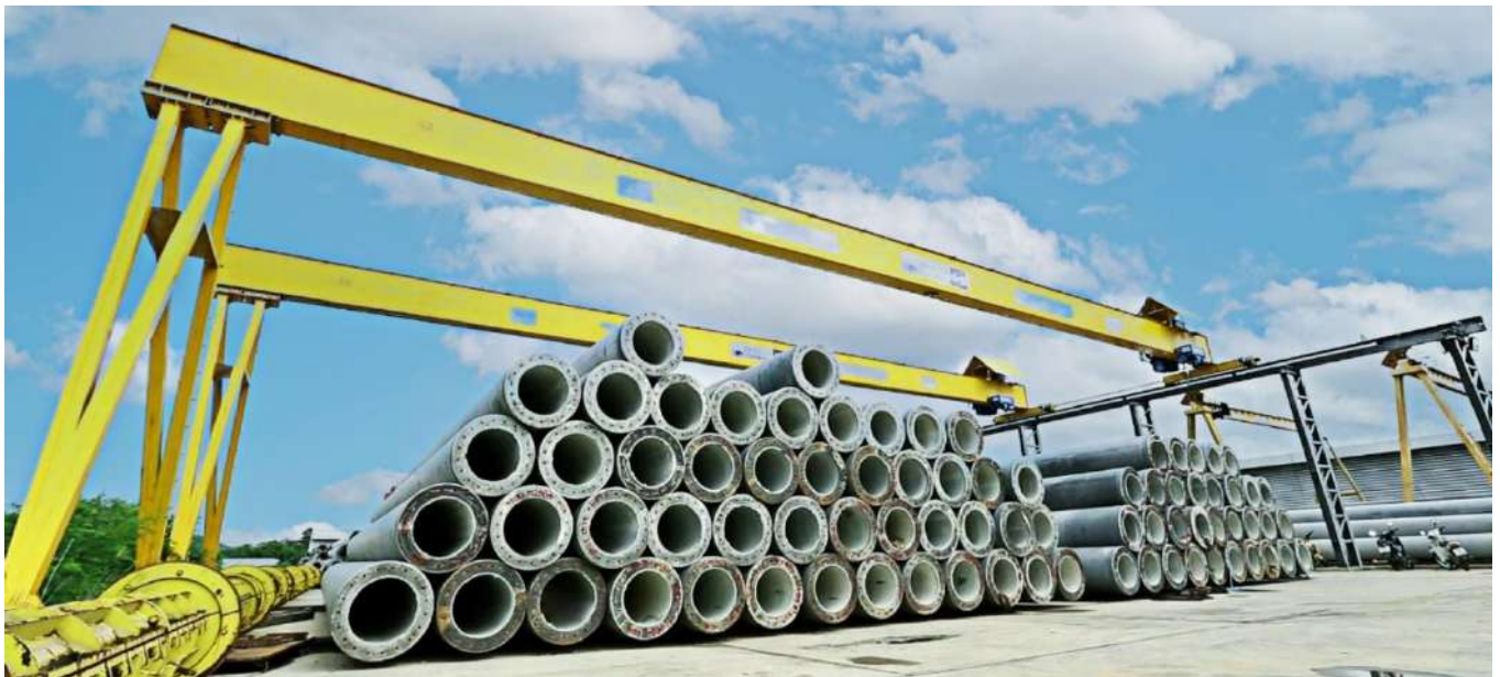
Example of the Company's spun pile
