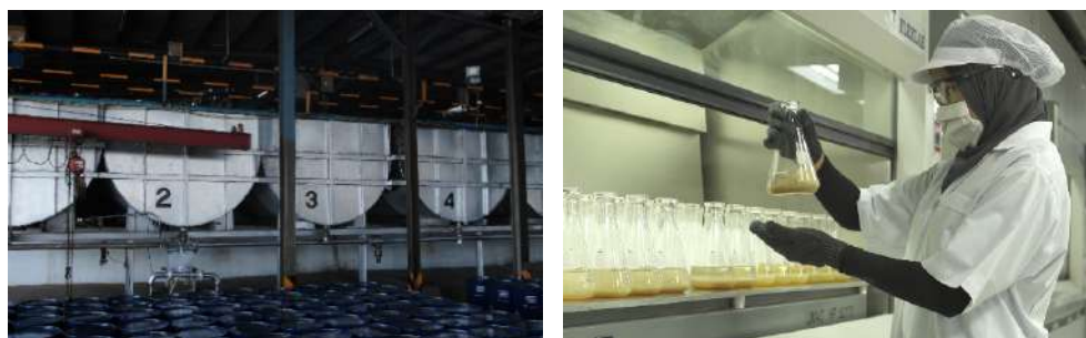
Mixing process and quality inspection of concentrated latex
