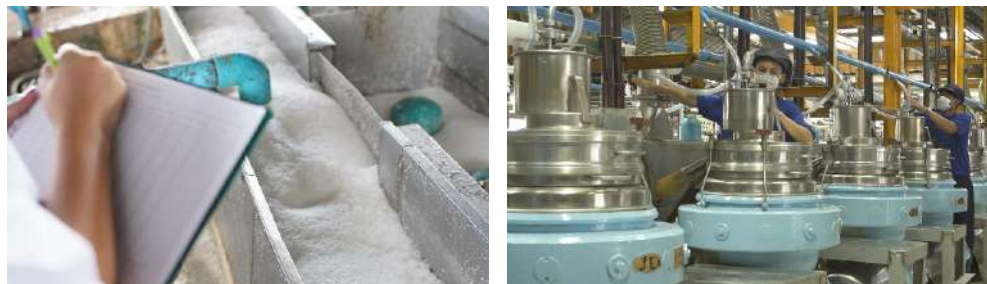
Quality inspection and contaminant removal process from field latex
