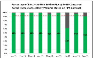
**TSG**, a 9.2 MW power plant selling electricity under the FiT system (4.47 baht/unit), generated and sold 19,398,325 units of electricity in Q3-2019 with thirteen hours of an unplanned shutdown. Details as follows.
